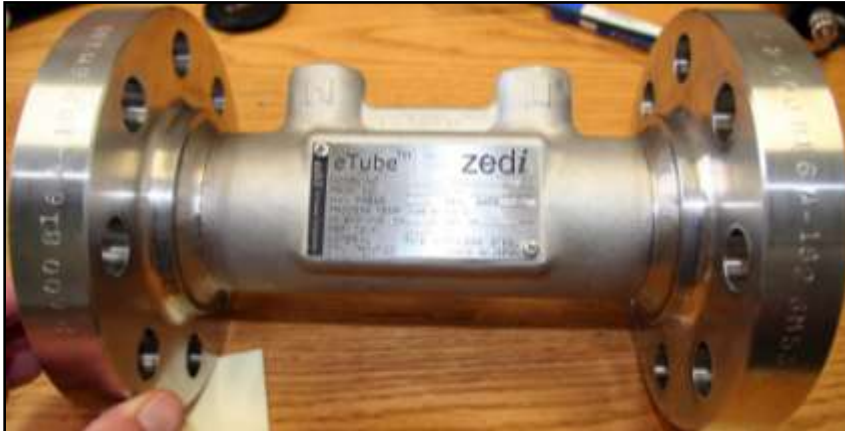
Figure 5: External condition of the eTube after removal
