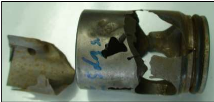
Figure 4: Damaged dump valve removed from pipe
