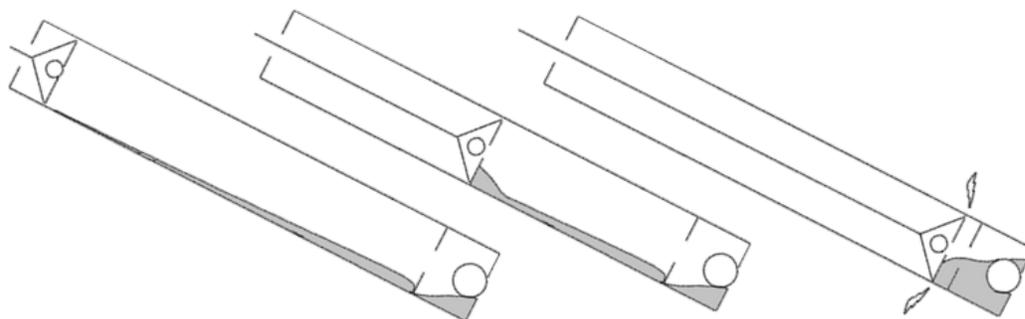
Figure 2, sand/debris accumulations
