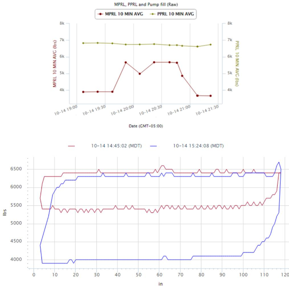
This is a well in northern North Dakota; the pump is landed at 3150ft (960m). Stuck open standing valve resulted in sudden increase in min polish rod load. In both Case 1A and 1B, resolution was a remote change in down stroke velocity (increased by about 1/3) for a period of about 30 minutes. Once cards returned to normal the initial down stroke velocity was restored.
