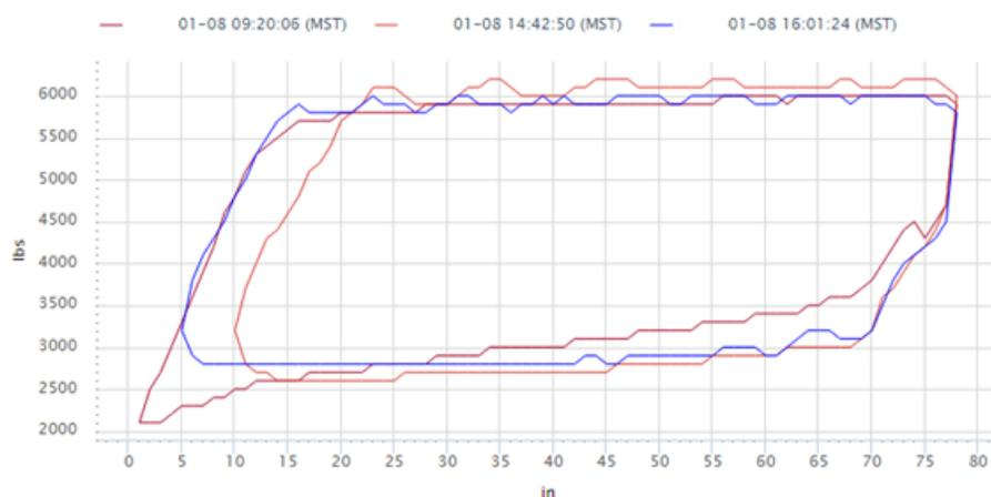
This is a well in south eastern Alberta; the pump is landed at 2723ft (830m). Sand entered pump and built up, the stroke was shortened and pump speed increased, then stroke length and rate restored, standing valve and pump now clear
