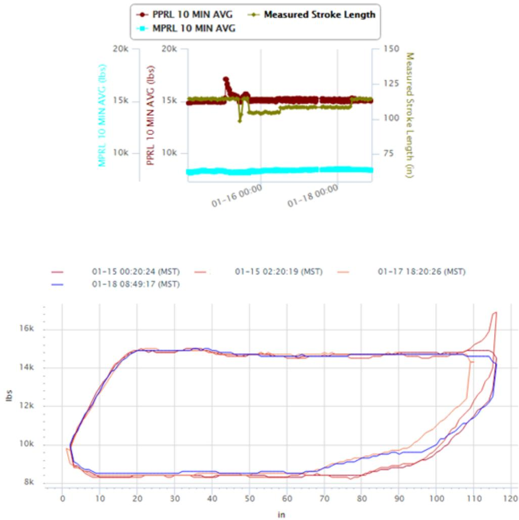
This is a well in south eastern Saskatchewan; the pump is landed at 4026ft (1227m). Sand accumulated at the top of the pump and caused plunger to have resistance at top of pump. The stroke length was lowered to stop compressing the sand. After a period of time, the sand got produced up the tubing and stroke length was restored.
