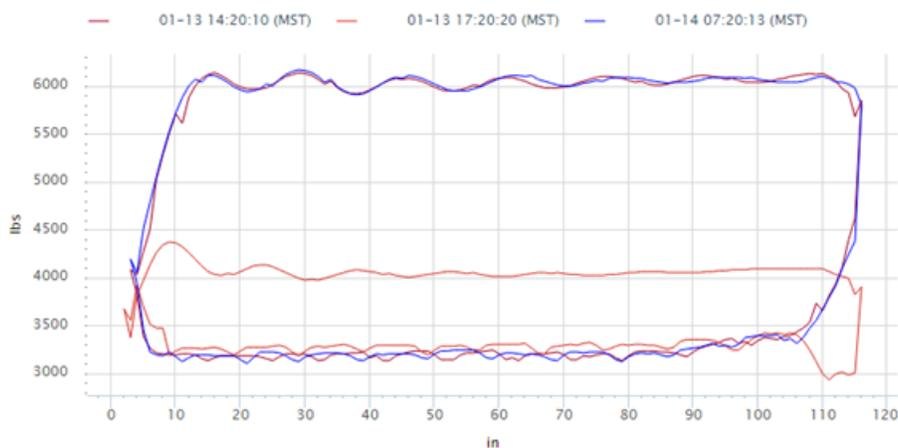
This is a well in south eastern Alberta; the pump is landed at 2560ft (780m). The travelling valve was not seating on the upstroke at 3spm. Increased upstroke speed and valve had proper sealing again. Cards shown: regular operation, non-sealing valve, back to regular operation
