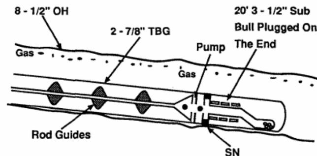
Figure 4, Typical setup for pumping a horizontal well in the deviated portion of the hole (Cortines, J. M. 1992)
