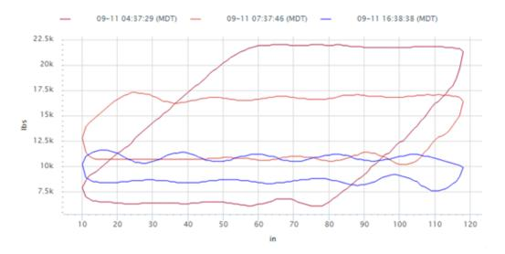
This is a well in northern Oklahoma; the pump is landed at 4780ft (1457m). The initial symptom was a sudden increase in min polish rod load followed by a steady decline in peak polish rod load. This is a classic sign of a stuck open standing valve where the traveling valve isn't opening and fluid is slowly lost due to slippage.
