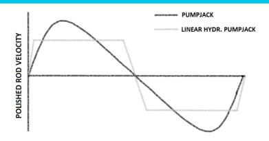
Figure 1, Polished rod velocity profiles of pump-jacks and linear hydraulic pump-jacks
