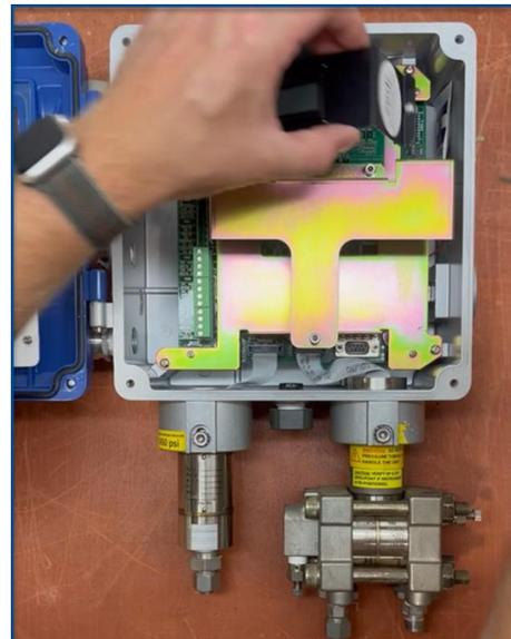
3. The SIM Card is in top right corner. Flip down the silver release, then pull up the SIM card with your fingers.
