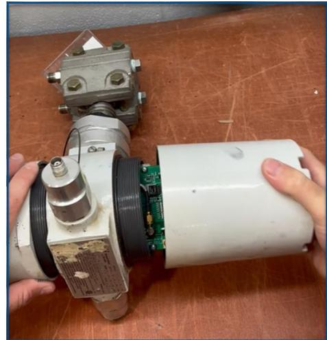
2. The SIM Card is located on the right. Loosen it with a screwdriver by pulling down on the tab.
