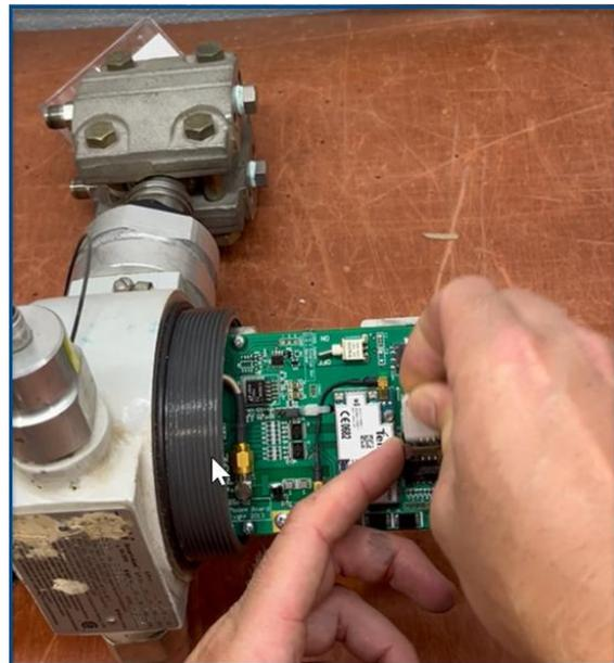
6. Reassemble the enclosure by twisting it back into place.
