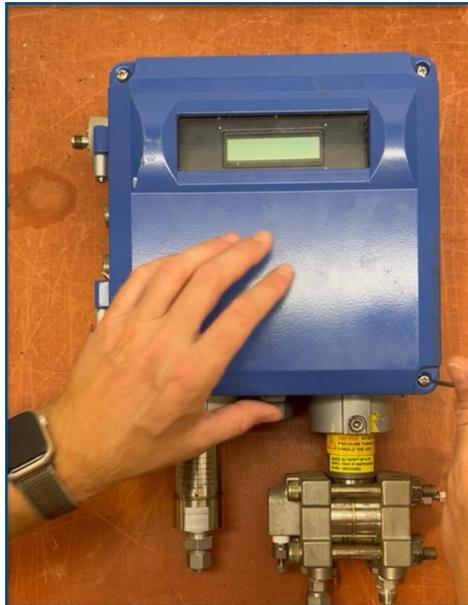
2. Locate the small screw to the right of the display and remove it using a Philips head screwdriver.
