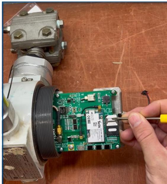
3. Pull up on the SIM holder and remove SIM Card.
