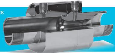
With its smooth shaped throat, the eTube is designed to produce stable differential pressure across a wide range of flows, while allowing particulates like sand, and other solids to easily pass through the restriction without excessive wear and damage.
