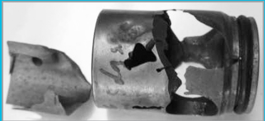
Figure 4: Damaged dump valve removed from pipe This resulted in the well being down for an additional period of time while the producer changed the downhole configuration. At this point, the producer removed the eTube for inspection, expecting significant wear given the damage incurred to the other pieces of equipment. In the time that the eTube had been installed, the severe levels of sand in the meter had chewed out two extra heavy flow joints at the well head and one dump valve (pictured in Figure 4).
